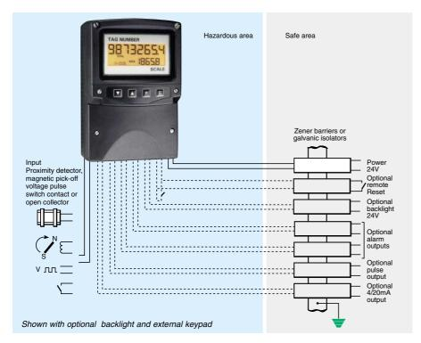
The BA334D is an externally powered, intrinsically safe rate totaliser with separate rate and total displays which will operate from a switch contact, voltage pulse, magnetic pick-off, open collector or a proximity detector input. A novel adaptive measuring technique plus an adjustable digital filter ensure that optimum rate display stability and step response can be achieved over a wide input frequency range.
